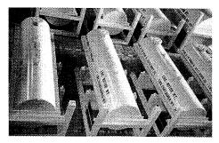
These canisters were flanged and linked in series for a dry air system and were used in transporting rotors between England and the Netherlands for a major overseas turbomachinery company.
